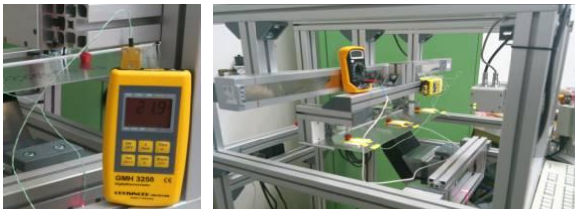
Figure 6 Image of the dual channel temperature meter GMH 3250 and the method of measuring the temperature during induction heating of the plate
