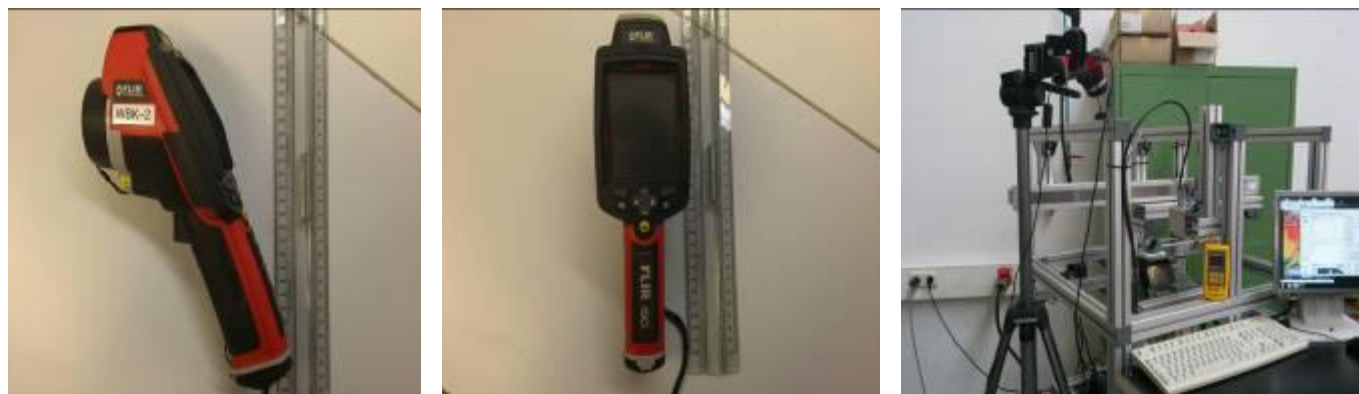
Figure 7 Image of the infrared camera i60, product of the firm Flir Systems GmbH and the example of the measurement of the temperature field
