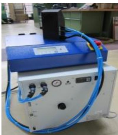
Figure 5 Image of the coaxial coil KI-112-U-30° with a pulse generator and chiller EW100W
