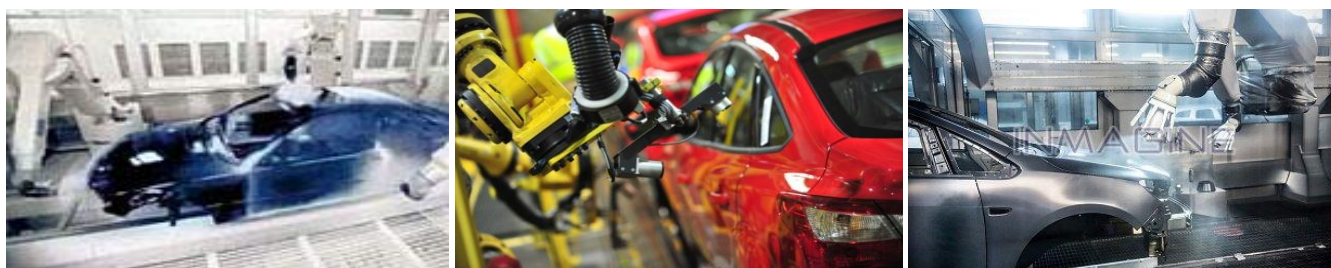
Fig. 12 Application of industrial robots in painting process and inspection of automobiles [3]
