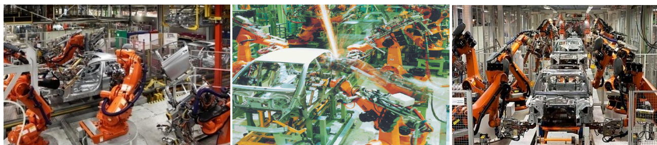
Fig.4 Industrial robots in welding process of automobile shell [20]
