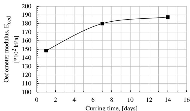
Fig. 7 Variation of oedometer modulus with curing time for (200 ÷ 300)kPa interval
