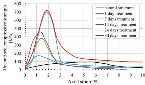
Fig. 5 Effect of curing time on unconfined stress-strain of the Bahlui clay
