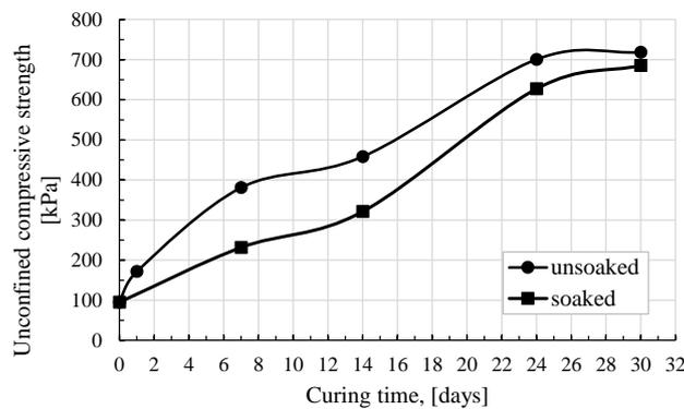
Fig. 6 Effect of curing time on unconfined stress-strain of the stabilized Bahlui clay with 10% cement
