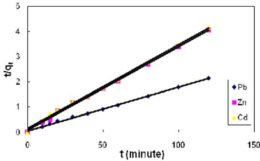
Fig. 6 Pseudo-second-order kinetics of biosorption of Pb(II), Zn(II), and Cd(II) onto loquat bark. Initial metal concentration 40 mg L<sup>-1</sup>; pH 4; at temperature 30 oC
