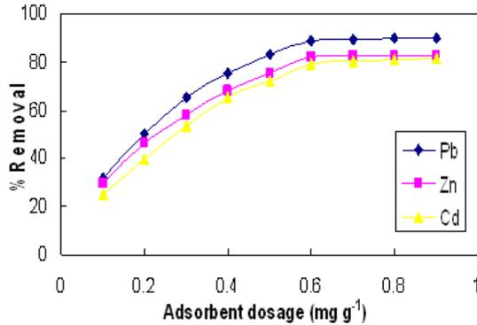
Fig. 3 Effect of biosorbent dosage on the biosorption of Pb(II), Zn(II), and Cd(II) onto loquat bark. Initial metal concentration 40 mg L<sup>-1</sup>; pH 4; at temperature 30 oC
