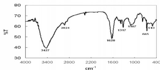
Fig. 1 FT-IR spectra of loquat bark before biosorption
