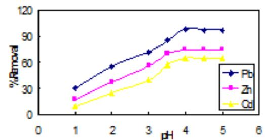
Fig. 2 Effect of pH on the biosorption of Pb(II), Zn(II), and Cd(II) onto loquat bark. Initial metal concentration 40 mg L<sup>-1</sup>; at temperature 30 °C
