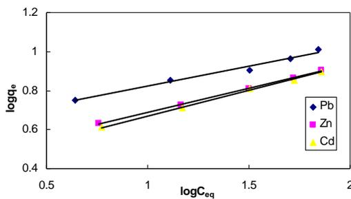
Fig. 8 The Freundlich isotherm plot for Pb(II), Zn(II), and Cd(II) adsorption on loquat bark; pH 4; at temperature 30°C
