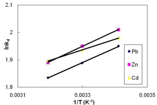
Fig. 11 Plot of  $\ln K_d$  vs.  $1/T$  for the estimation of thermodynamic parameters for biosorption of Pb(II), Zn(II), and Cd(II) onto loquat bark; pH 4
