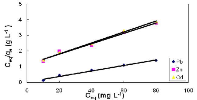
Fig. 7 The Langmuir isotherm plot of biosorption of Pb(II), Zn(II), and Cd(II) onto loquat bark; pH 4; at temperature 30 oC
