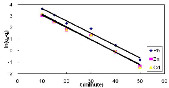
Fig. 5 Pseudo-first-order kinetics of biosorption of Pb(II), Zn(II), and Cd(II) onto loquat bark. Initial metal concentration 40 mg L<sup>-1</sup>; pH 4; at temperature 30 °C
