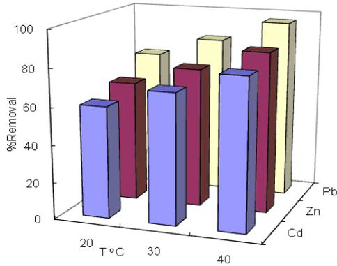
Fig. 10 Effect of temperature on the biosorption of Pb(II), Zn(II), and Cd(II) onto loquat bark; pH 4
