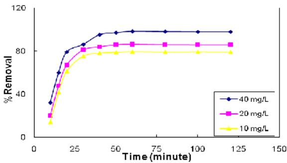
Fig. 4 Effect of initial concentration on the biosorption of Pb(II) onto loquat bark; pH = 4.0; at temperature 30 oC
