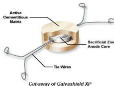
Fig. 2 Cut away section of anode
