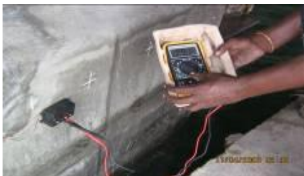
Fig. 11 Typical view of half cell measurement after rehabilitation
