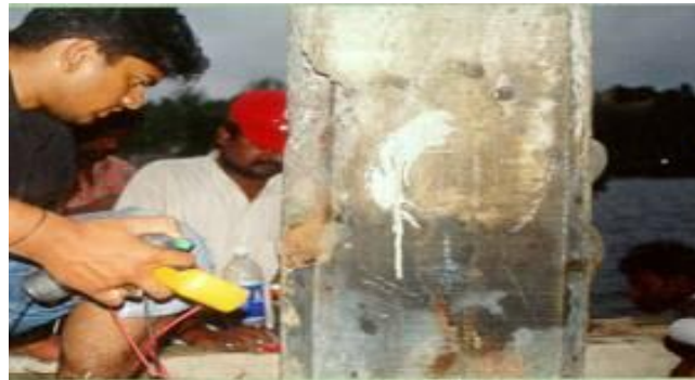
Fig. 3 Typical view of onsite measurement of half cell test
