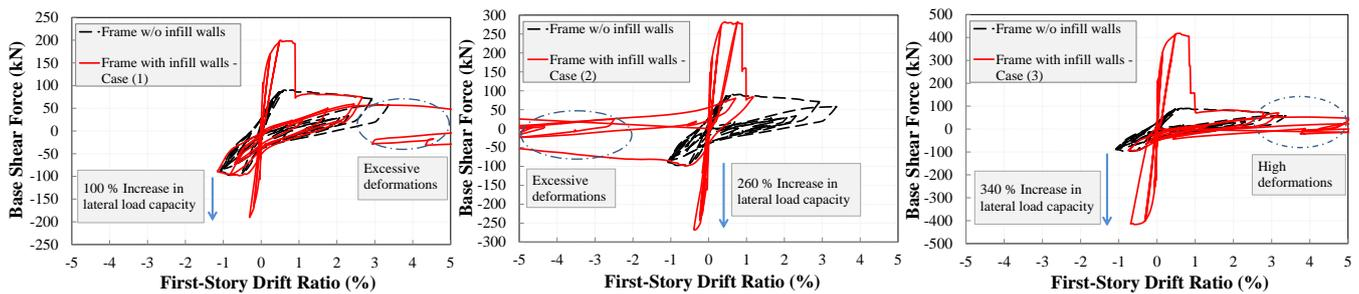
Fig. 9 Base shear versus top-story drift ratios with and w/o infill walls
