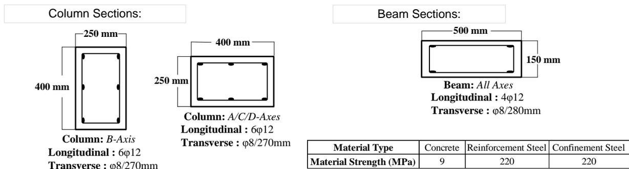
Fig. 5 Beam and column sections
