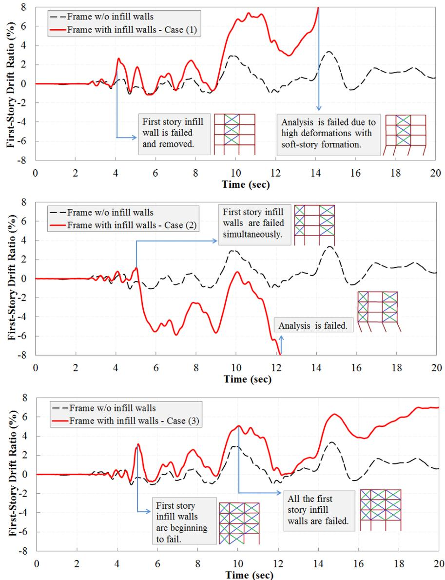
Fig. 8 Comparison of drift ratio results with and w/o infill walls
