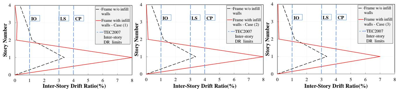
Fig. 10 Comparison of inter-story drift ratios with limit states
