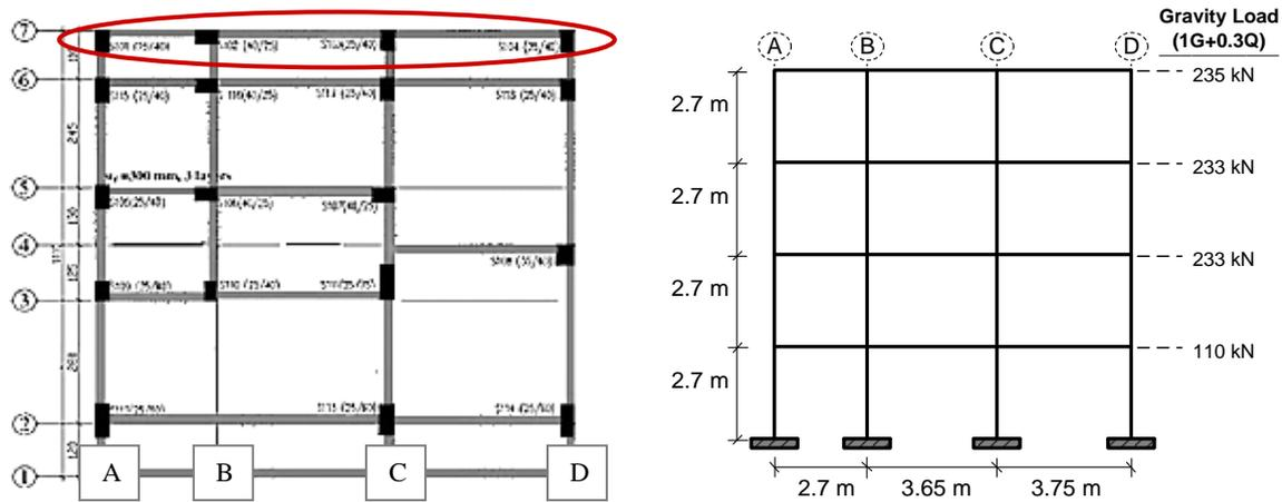
Fig. 4 Plan of the structure and tested frame
