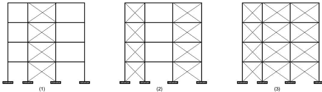
Fig. 6 Examined infill wall layouts
