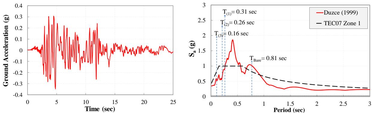
Fig. 7 Duzce ground motion and its spectrum
