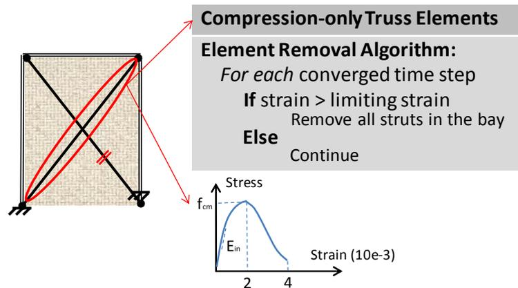
Fig. 3 Modelling of infill walls with element removal algorithm
