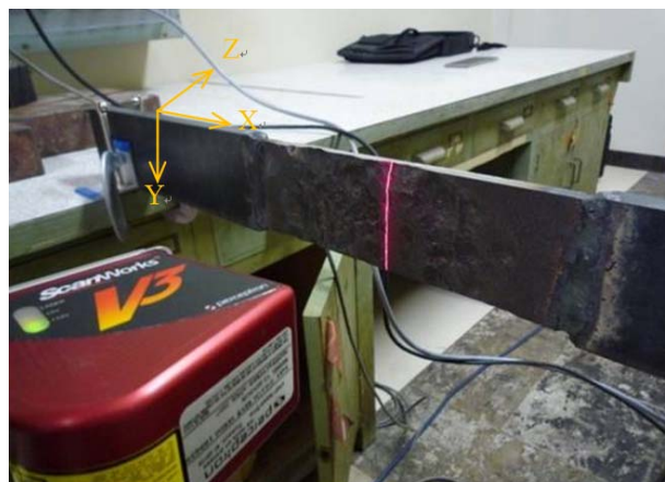
Fig. 2 Condition of thickness measurement
