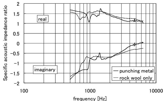
Fig. 11 Specific acoustic impedance ratio ( $\phi 29$ )
