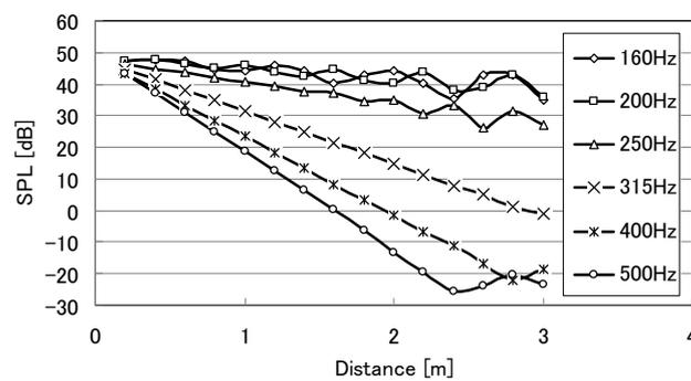
Fig. 12 Noise reduction with distance (W270H400)
