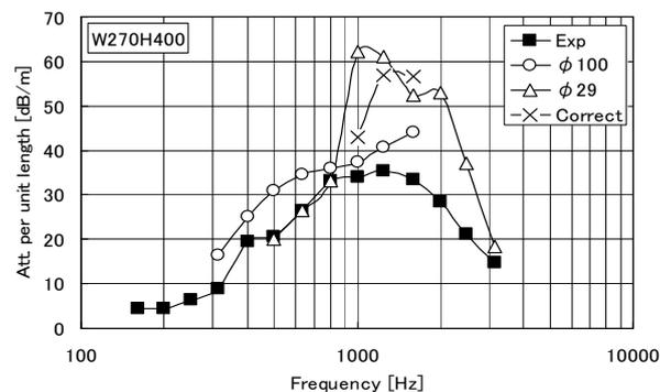
Fig. 14 Attenuation per unit length (P/S=18.4)
