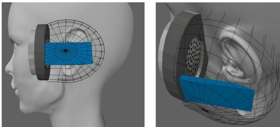
Fig. 1C The azimuth was controlled by a 40×30×1 mm plastic strip (indicated by the shaded rectangle) attached to the base of the speaker at a 10 degree angle. The strip served as a guide and reverberation surface for sound waves reaching from the speaker to the top of the external ear canal.
