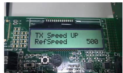
Figure 8 Motor speed-up by pushing button S5 (from Explore 16 EVB)
