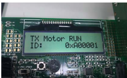
Figure 6 Motor start by pushing button S3 (from Explore 16 EVB)
