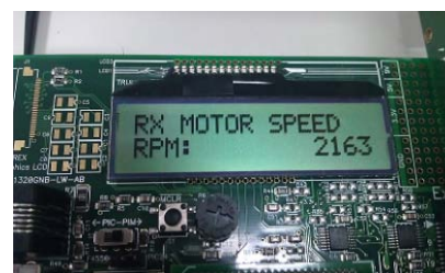
Figure 10 The status of motor speed responded (from dsPICDEM MCLV )
