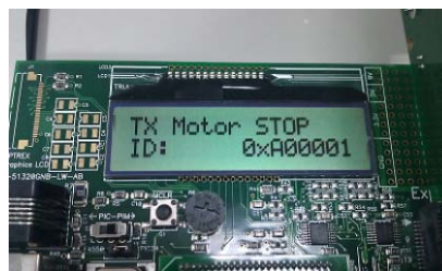
Figure 7 Motor stop by pushing button S6 (from Explore 16 EVB)
