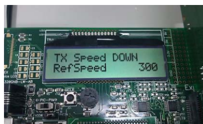
Figure 9 Motor speed-down by pushing button S4 (from Explore 16 EVB)
