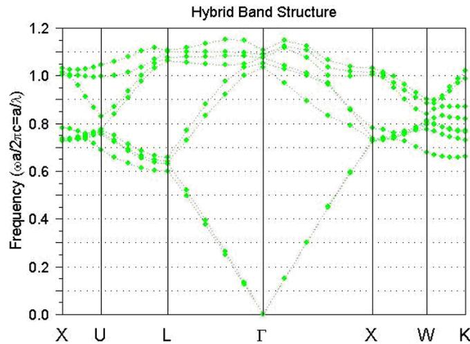
Fig. 1 Energy band diagram of the FCC structure colloidal crystal fabricated by SiO<sub>2</sub> microspheres
