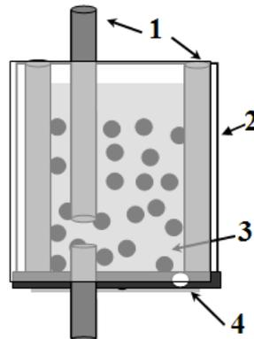
Fig. 2 Diagram of the device to fabricate colloidal crystals
