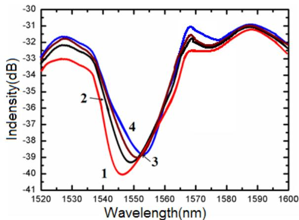
Fig. 5 the transmittance spectra of colloidal crystals immersed in the different liquid materials (1. pure water, 2. pure water with the acetone(1:1), 3. 2. acetone with the pure water (1:2), 4. acetone)
