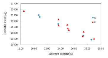
Figure 3 Relationship of calorific value versus moisture content
