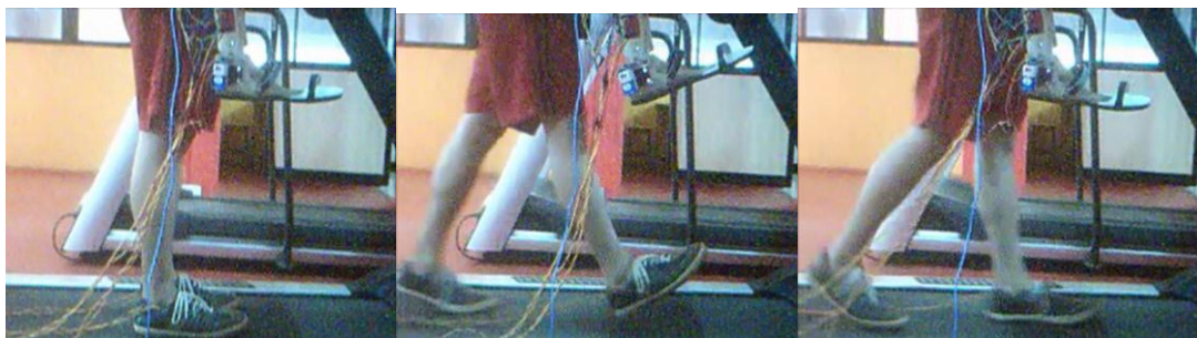
Fig.10 Treadmill testing of the device showing planar and dorsi assist for the right foot.
