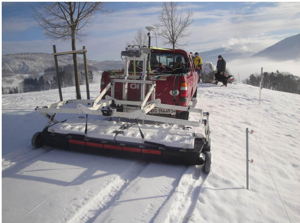
Fig. 1 The STREAM X system. White boxes (back of the car) contain an array of 15 antennae. A hydraulic mechanical system allows lifting the antenna boxes up and down in order to assure good ground-coupling and to avoid obstacles.
