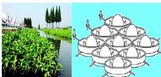
Fig. 7 Bouyant material AFIs designed by Hubei University (Material is comprised of polyester fibre matrix injected with polystyrene foam to form a floating platform).
