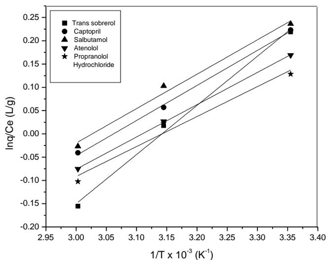
Fig. 11 Van't Hoff plot for R-isomers of racemic compound on polymer 3
