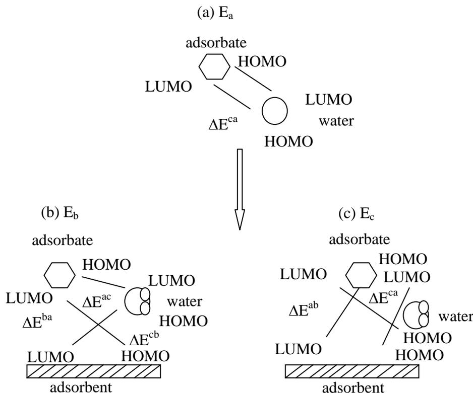
Fig. 5 Three body interaction model
