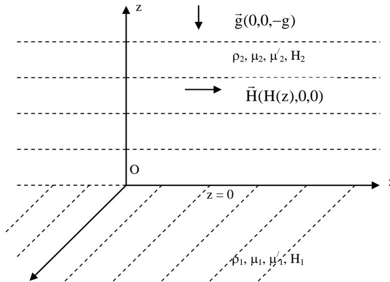
Fig. 1 Two uniform Rivlin-Ericksen elastico-viscous fluids separated by a horizontal boundary  $z = 0$
