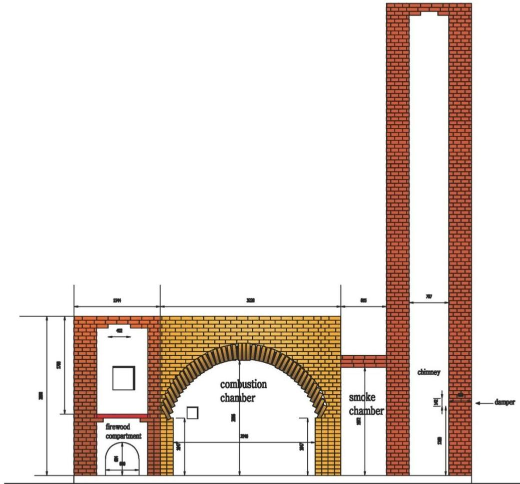
Fig. 4 Cross section of the re-designed kiln showing main combustion chamber, smoke retention chamber, and firewood stoking chamber
