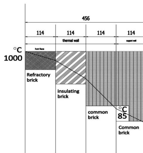
Fig. 1 A schematic representation of the kiln wall with the inner wall servicing 1000 °C and the outer servicing 85 °C
