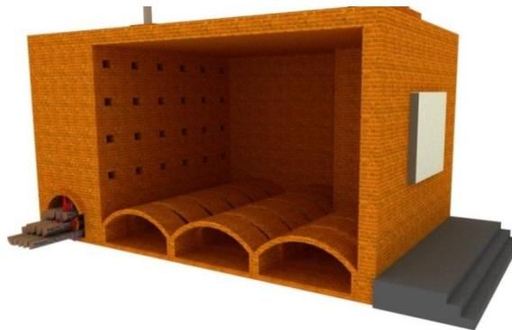
Fig. 3 Perspective view showing novelty in design of the fixed arches with refractory bricks and fire wood heat generating chamber
