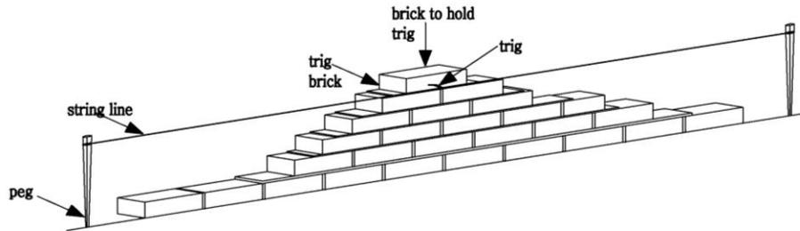
Fig. 2 Technique for laying arrangement of the brick wall construction
