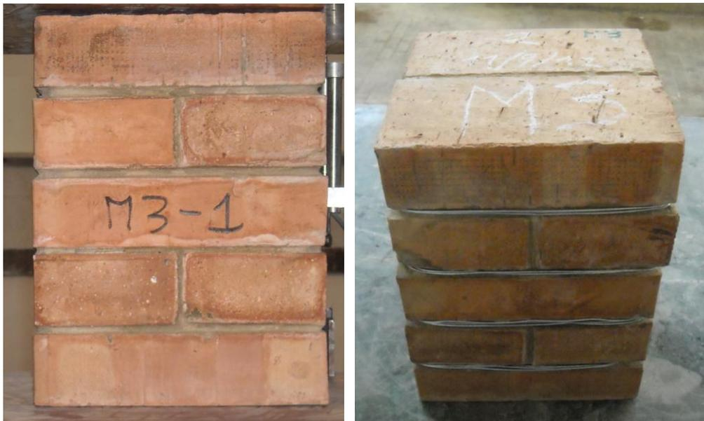
Fig. 2 Solid brick masonry columns: a) unconfined; b) confined with steel wires
