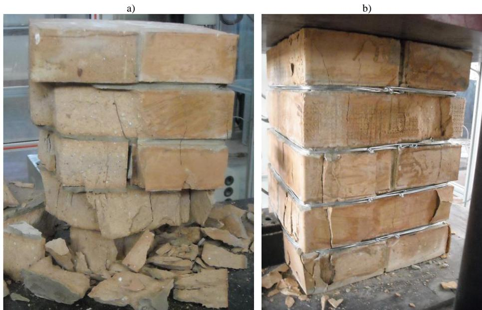
Fig. 7 Failure modes of masonry columns. a) Unconfined; b) confined
