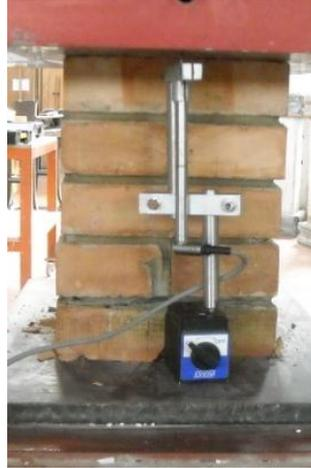
Fig. 5 Compression tests on masonry columns
