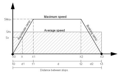
Fig. 3 UPTS speed vehicle ramp.
