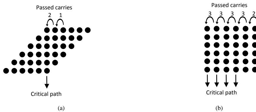
Fig. 7 Critical path of (a) 6x6 multiplication, (b) 6x6 CSA array
