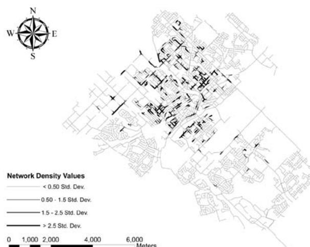
Fig. 4 Density estimation of inspected pipes found to be in bad condition (ICG 4-5)
