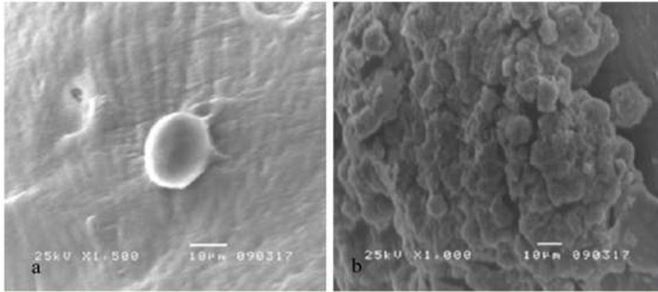
Fig. 6 MNCs attachment on the scaffold surface were imaged by SEM after 2 week culturing ((a): one cell, (b): cell cluster)
