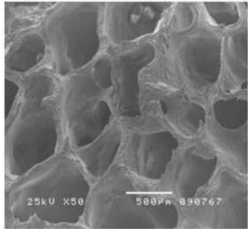
Fig. 2 The SEM result for identifying the spongy structure of the decellularized bone. The pore sizes were about 250-1000  $\mu\text{m}$ . Distance between 2 pores is 50-100  $\mu\text{m}$
