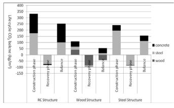
Figure 3. Life cycle CO<sub>2</sub> balance of structures.
