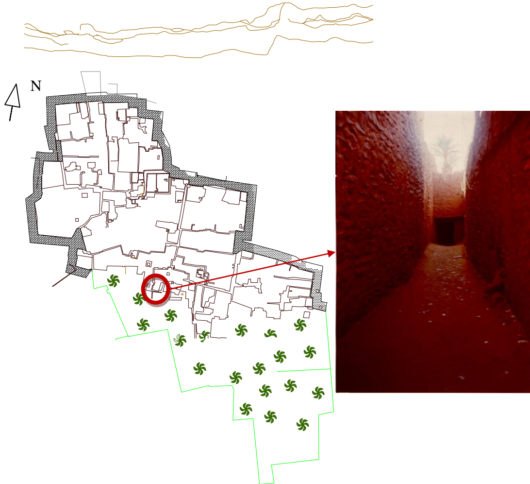
Fig. 4 Shadow effect at the level of the alleys, of the vernacular establishment, result of a narrow and twisty configuration. Example: Kenadsa' ks ar
