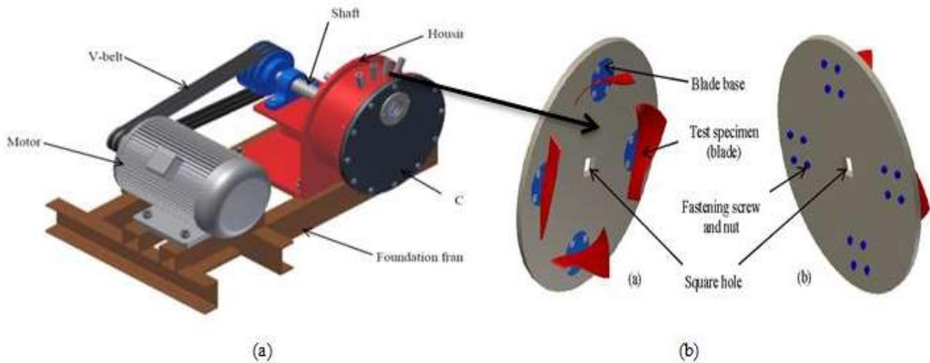
Fig. 1 (a) Rotating disc apparatus for erosion test (b) Position of test specimen [9]
