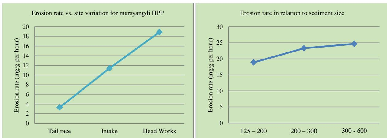
Fig. 4 Erosion analysis graphs
