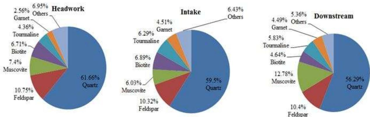
Fig. 3 Pie chart representing the mineral analysis of the Marsyangdi HPP
