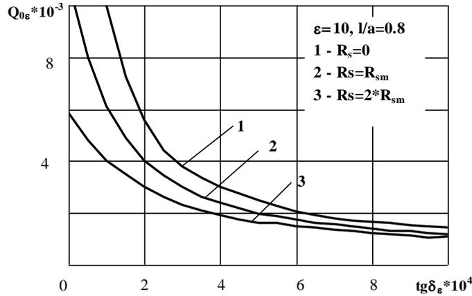
Fig. 2  $Q_0$ -factor value dependence of  $H_{011}$ -mode of cylindrical-radial waveguides junction with a disk on superficial resistance value  $R_s$
