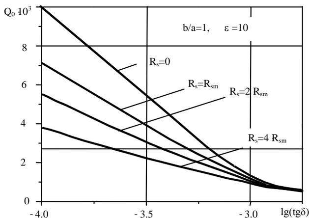
Fig. 4 Dependence of eigen  $Q_0$  -factor value of  $H_{110}$  -mode on loss tangent for various values  $R_s$  ( $R_{sm}$ - superficial resistance of copper)
