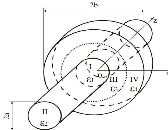
Fig. 1 Junction of cylindrical-radial waveguides
