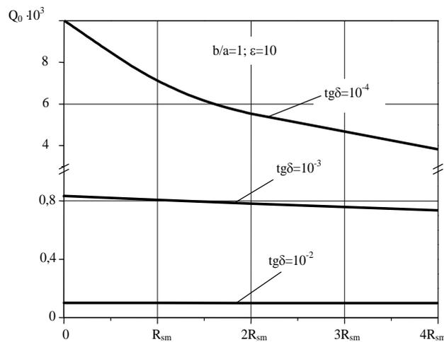
Fig. 5 Dependence of size of eigen  $Q_0$ -factor value of  $H_{110}$  -mode on superficial resistance value  $R_s$
