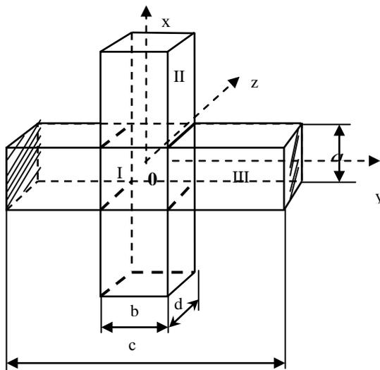
Fig. 3. Junction on rectangular waveguides
