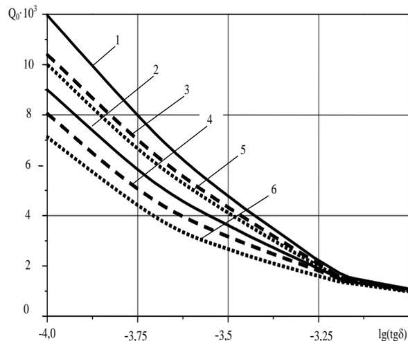
Fig. 6 Dependence of eigen  $Q_0$ -factor value on loss tangent  $\text{tg}\delta$  for various types of junctions, loaded with dielectric:  $\epsilon=10$ ;  $b/a=1$ ; curves 1 and 2 - junction of cylindrical - radial waveguides, (1 -  $R_s=0$ ; 2 -  $R_s=R_{sm}$ ); curves 3 and 4 - junction of cylindrical - rectangular waveguides, (3 -  $R_s=0$ ; 4 -  $R_s=R_{sm}$ ); curves 5 and 6 - junction on rectangular waveguides (5 -  $R_s=0$ ; 6 -  $R_s=R_{sm}$ )
