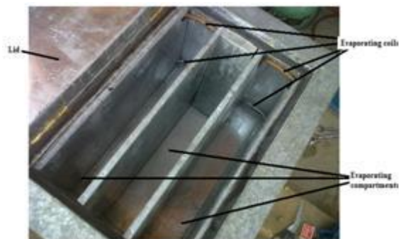
Fig. 3 The refrigerating box opened showing, the refrigerating space with compartments; the compartments houses the evaporating coils
