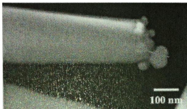
Fig. 4 The SEM of surface in one array of Ag/ZnO
