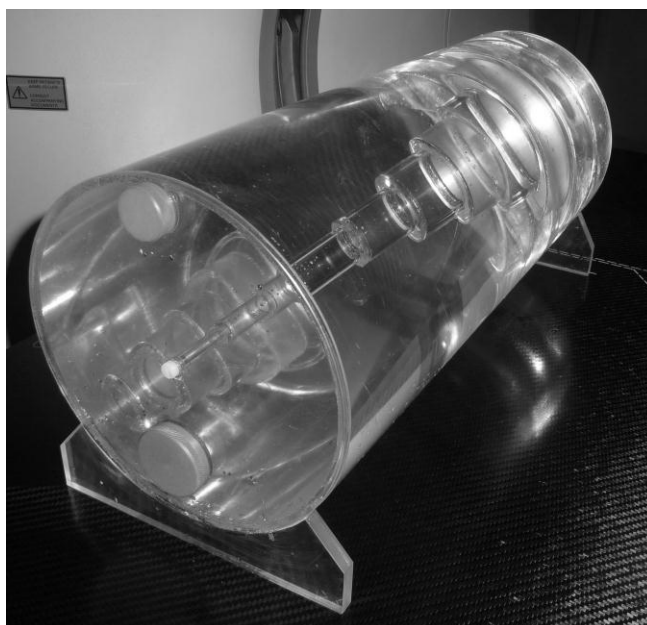
Fig. 1 In-house constructed phantom with eight connected inner cylinders
