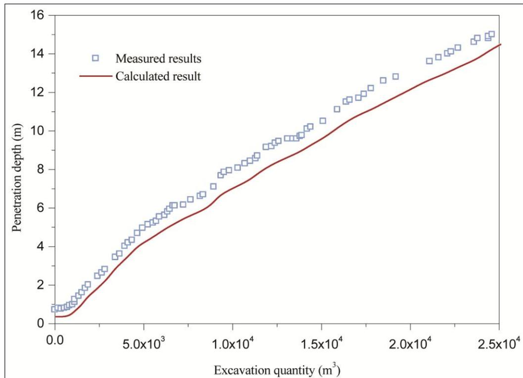
Fig. 8 Penetration depth varying with the quantity of excavation
