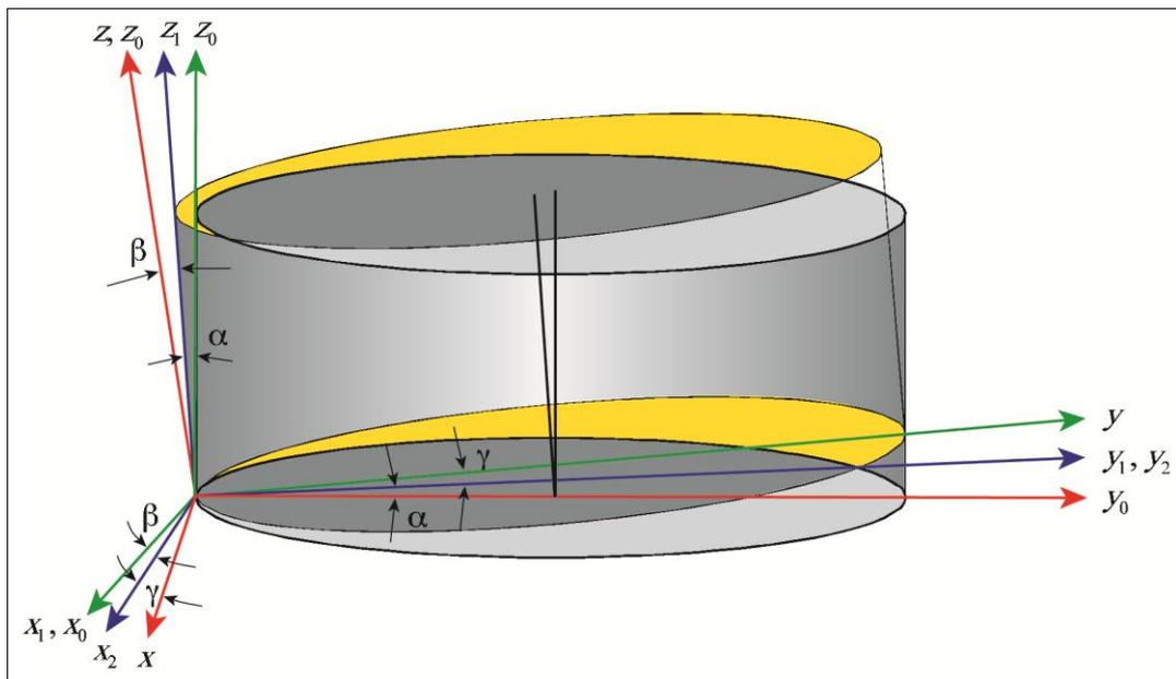
Fig. 4 Deflection of the extra caisson during the penetration
