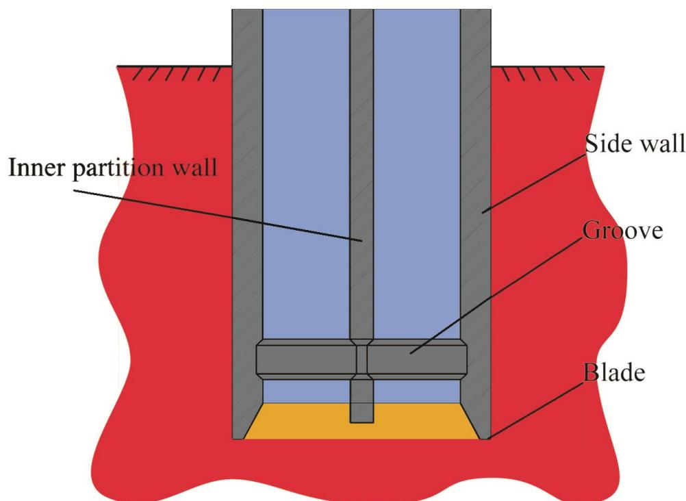
Fig. 1 Schematic diagram of a large extra concrete caisson
