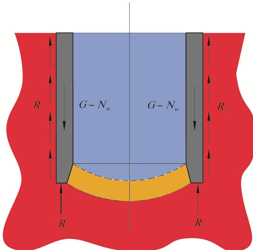
Fig. 2 Main loads distribution on the large extra concrete caisson
