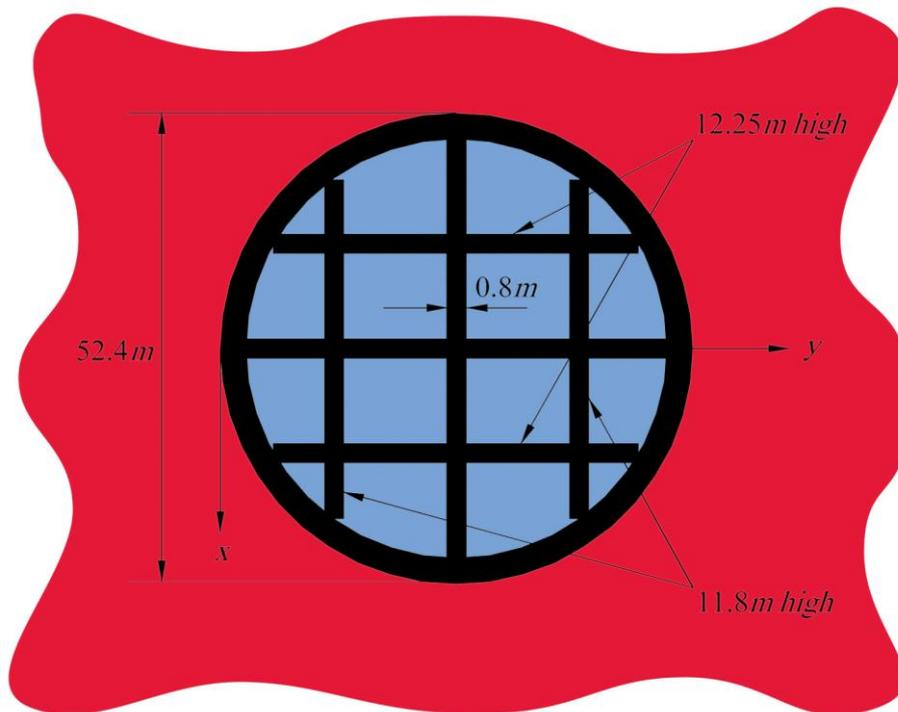
Fig. 6 Layout chart of the extra caisson in the site
