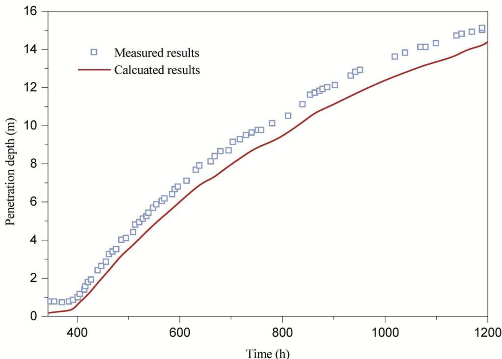
Fig. 7 Time history of the extra caisson penetration depth
