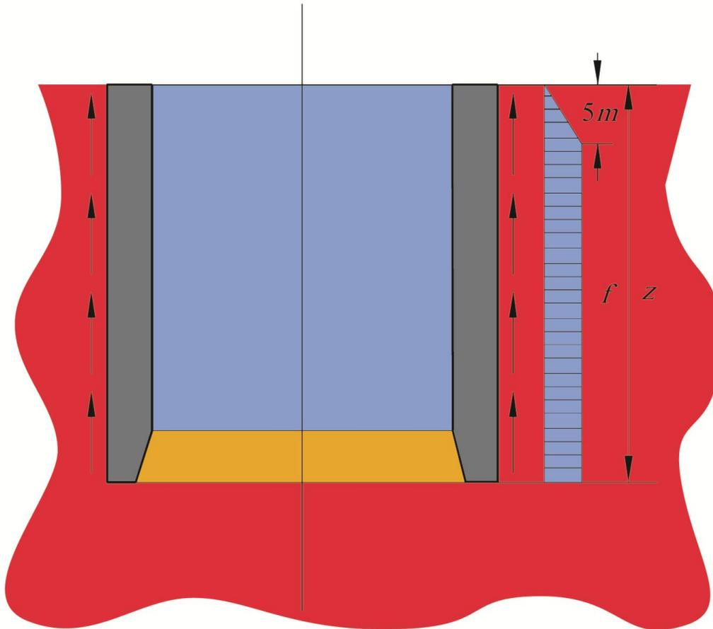
Fig. 3 Unit area lateral friction distribution along the wall
