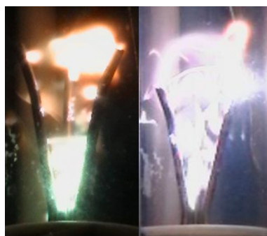
Fig. 7 (a) Plasma formed with only argon; (b) plasma formed with acetone and argon
