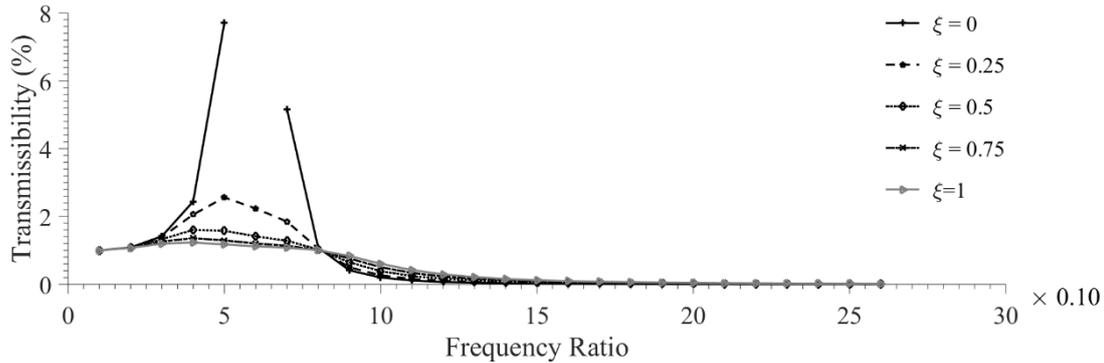
Fig. 4 Theoretical Frequency Response of a Man/Seat Model for Five Levels of Damping Ratios
