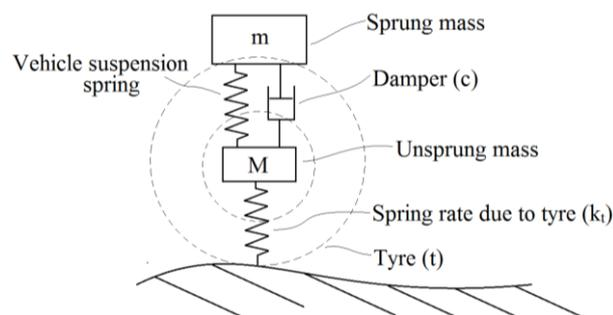
Fig. 1 Suspension of a Work Vehicle on a Terrain with Sinusoidal Cross-Section
