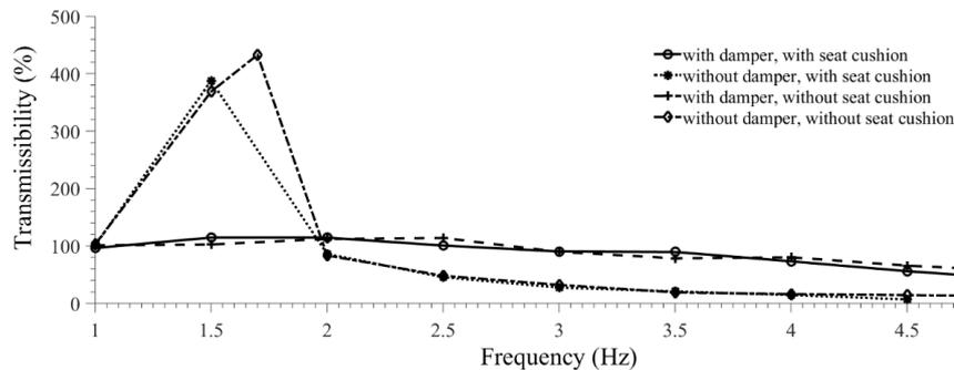
Fig. 8 Transmissibility of Seat at Input Amplitude  $X = 12.5\text{mm}$
