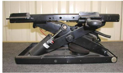
Sample Scissors Seat Mechanism with Damper, Pneumatic Suspension and Spring
