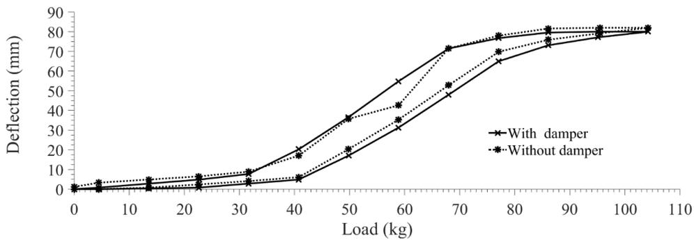
Fig. 5 Load – Displacement Curves for the Suspension Seat Mechanisms
