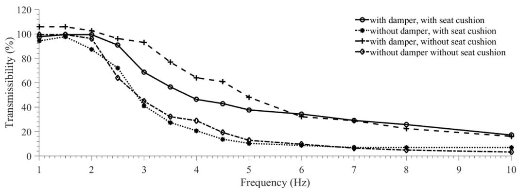
Fig. 7 Transmissibility of Seat at Input Amplitude X = 6.25mm
