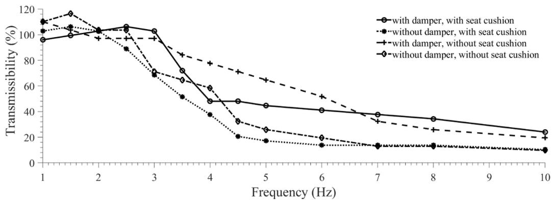
Fig. 6 Transmissibility of Seat at Input Amplitude X = 3.12mm
