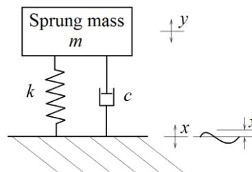
Fig. 3 Simplified Man/Seat Model Subjected to Vibrations
