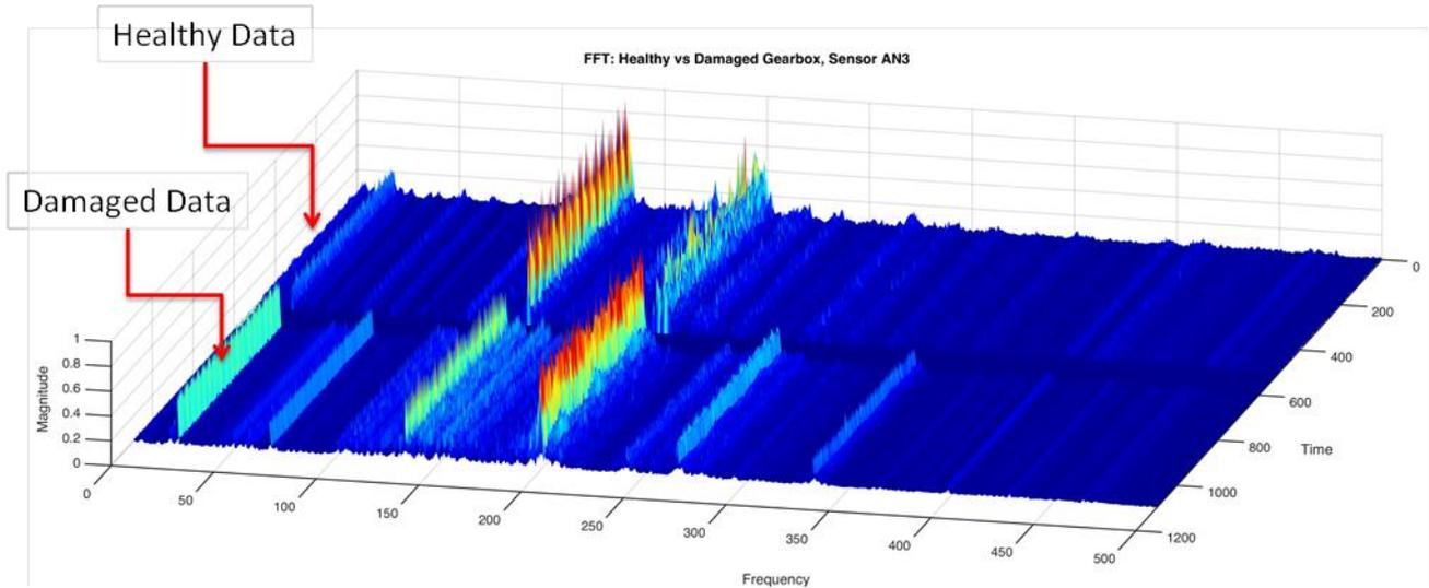
Fig. 10 Plotting healthy FFT data against damaged data
