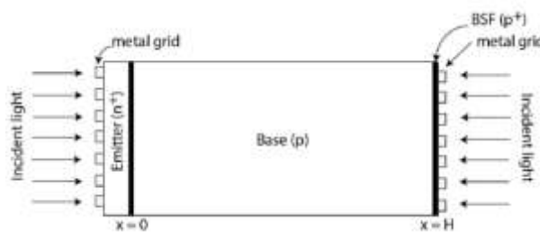
Fig. 1 Bifacial silicon solar cell
