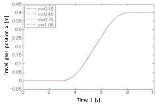
Fig. 6 Travel gear position for load mass change in the model
