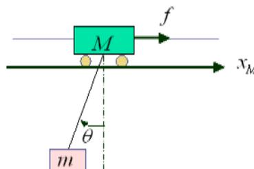
Fig. 1 Overhead travelling crane physical model
