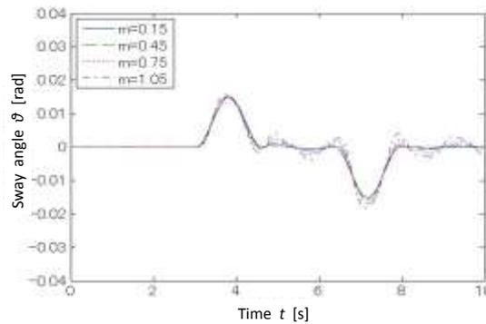
Fig. 7 Sway angle for load mass change in the model
