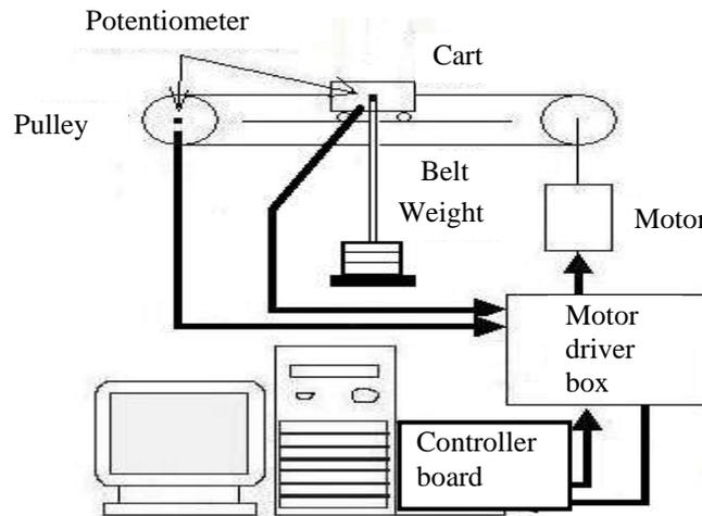
Fig. 8 Control system configuration
