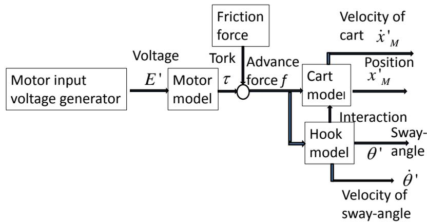
Fig. 2 Reference model configuration
