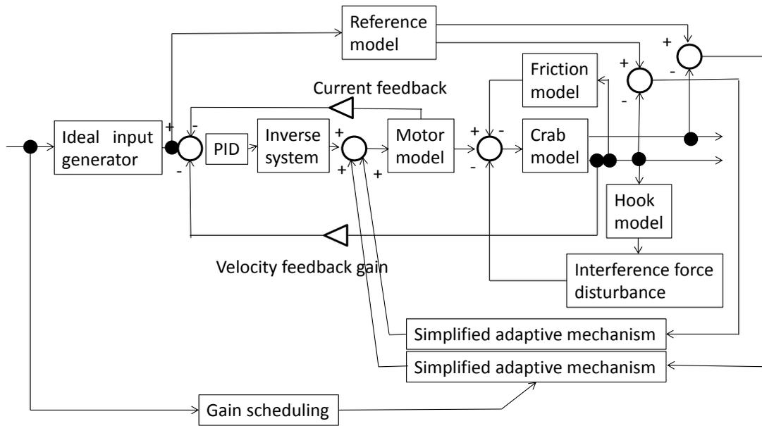
Fig. 5 Configuration of MRSACS for a crane with crab
