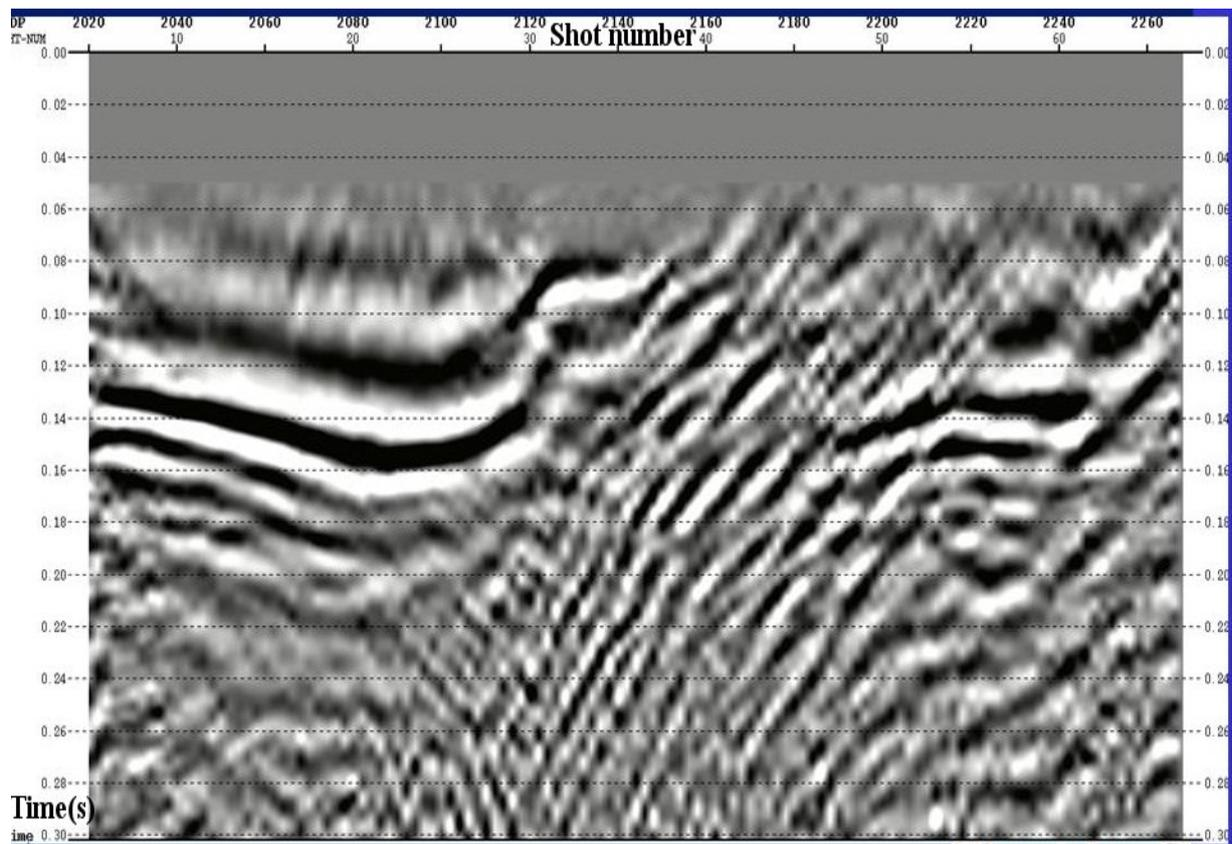
Fig. 5 CMP stacked section obtained using conventional processing
