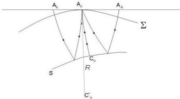
Fig. 1 Schematic description of the ray path from reflector S
