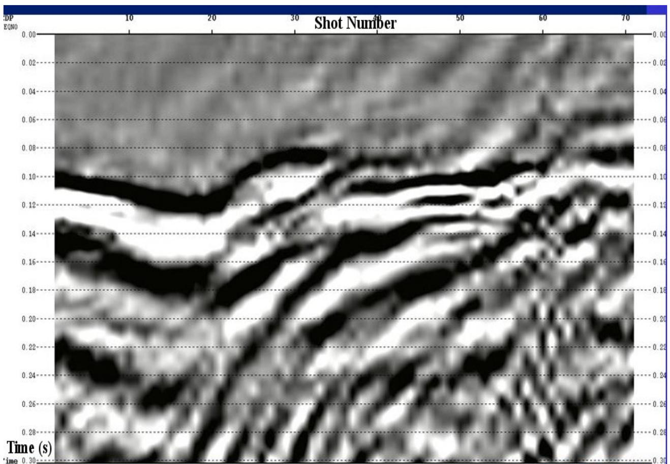
Fig. 6 CSP time section obtained using the weighted multipath summation
