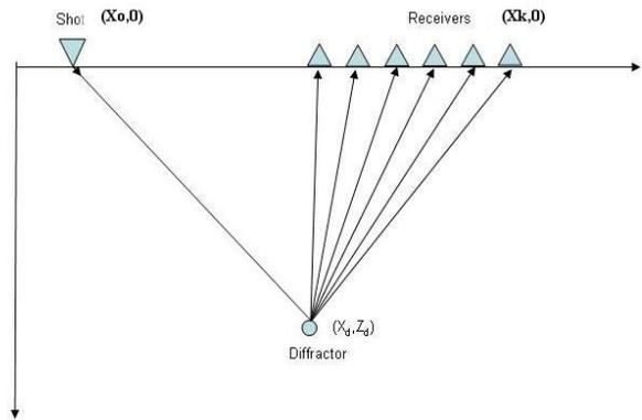
Fig. 2 Schematic description of the ray path from diffractor  $X_d, Z_d$
