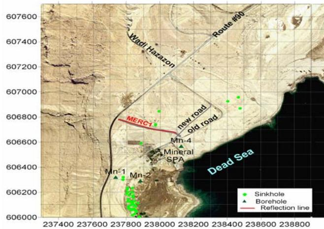
Fig. 3 Mineral Beach (Shalem-2) sinkhole development area with location of the MERC1 seismic reflection line
