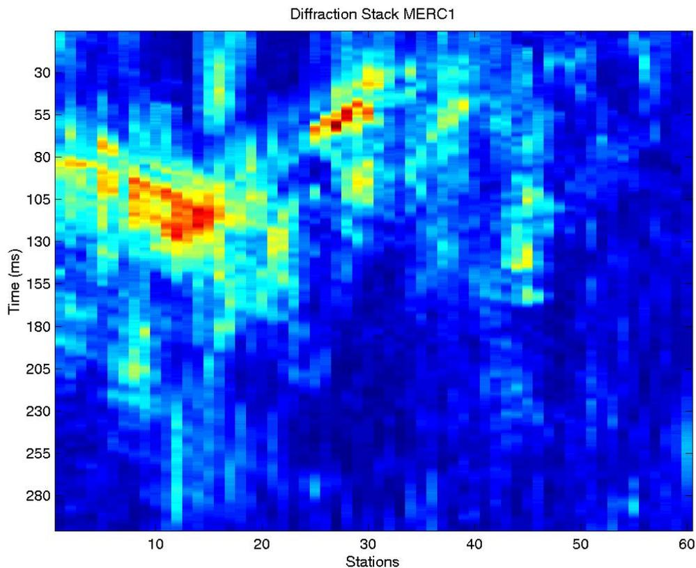
Fig. 7 Diffraction image obtained by diffraction method using weighted multipath summation
