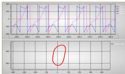
Figure 14 Trajectory of saddle (top) and motor (bottom) on the experiments
