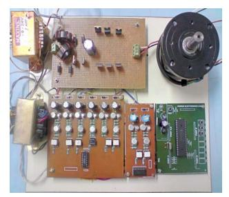
Fig. 7 (a) Hardware of Bridgeless boost converter fed BLDC motor
