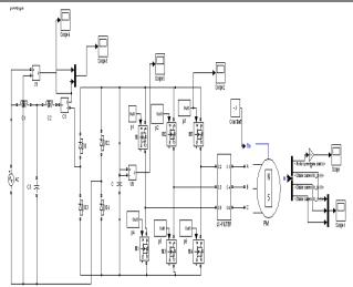
Fig. 4 (a) VSI with input T-filter fed BLDC motor
