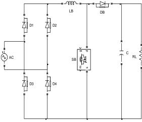
Fig. 2 Conventional PFC boost rectifier
