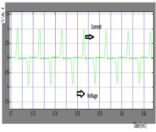
Fig. 4 (b) Input current waveform
