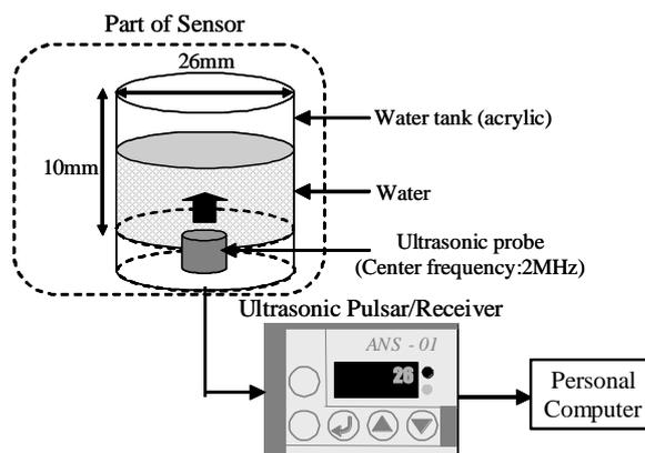
Fig. 3 Ultrasonic Oscillosensor system
