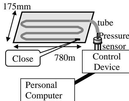
Fig. 2 Air pressure sensor system
