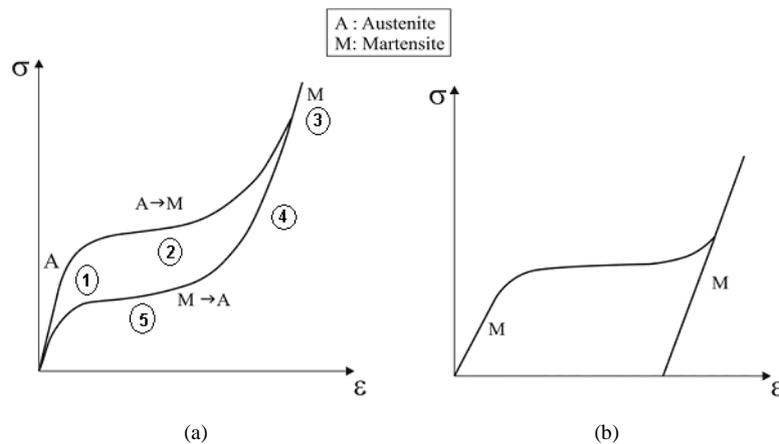
Fig. 1 Stress-strain curves for SMAs: (a) superelasticity effect; (b) shape memory effect [13]
