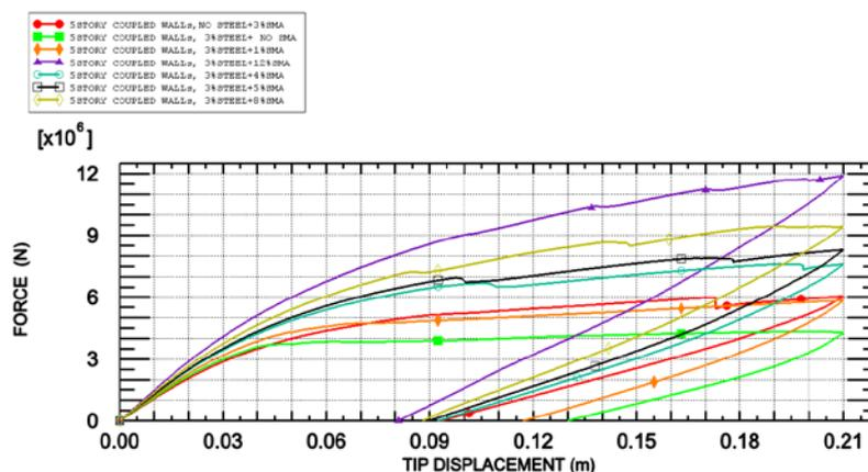
Fig. 10 Behavior of concrete shear wall with different percent of SMA reinforcements
