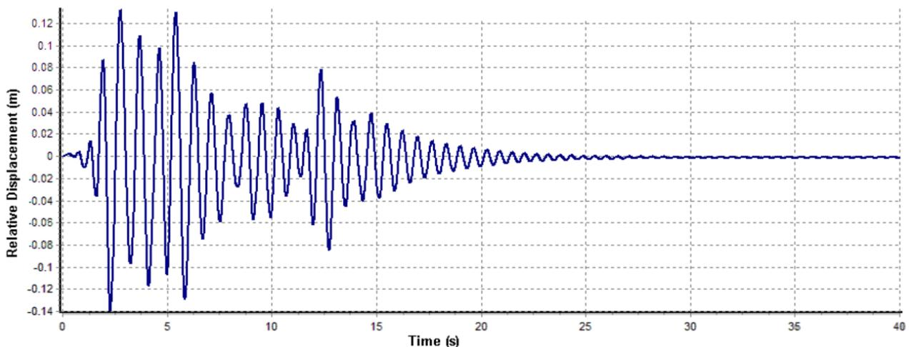
Fig. 4 Tip deflection response of structure with SMA bracings
