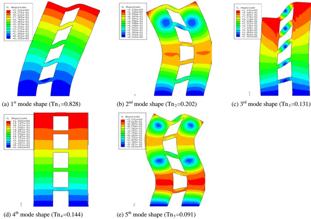
Fig. 9 Mode shapes of the shear wall
