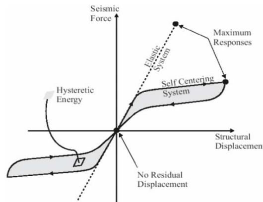
Fig. 7 Idealized Seismic Response of Self-Centering Structures [24]
