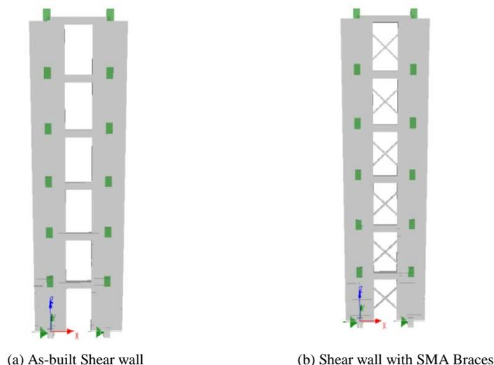
Fig. 2 Analytical models of the shear wall in SeismoStruct software
