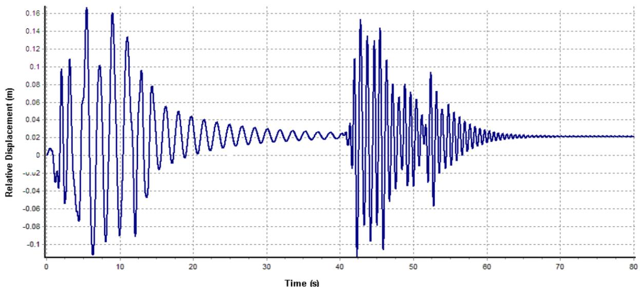
Fig. 6 Tip deflection response of structure with SMA repairing members in two stages
