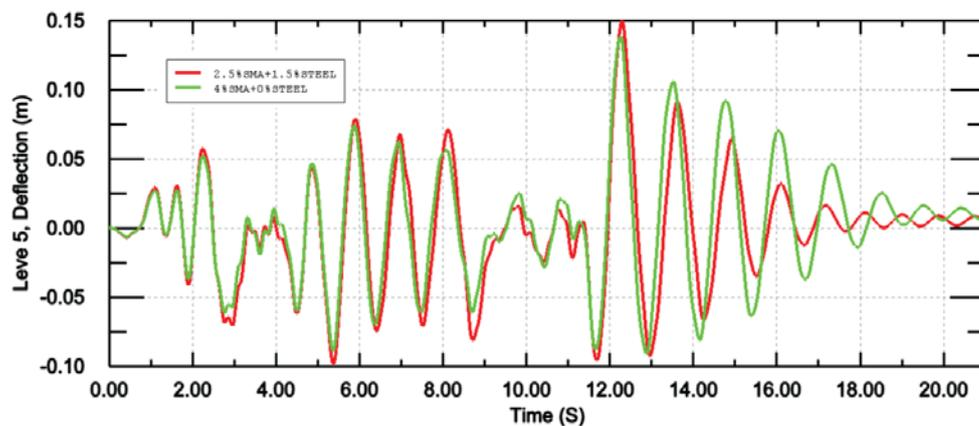
Fig. 12 Tip deflection of the shear wall subjected to El-centro earthquake for two different percentages of steel and SMA reinforcement
