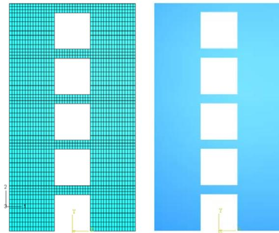
Fig. 8 Finite Element model of the reinforced concrete shear wall
