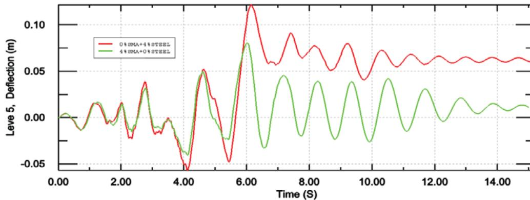
Fig. 11 Tip deflection of the shear wall subjected to Koyna earthquake for steel or SMA reinforcement
