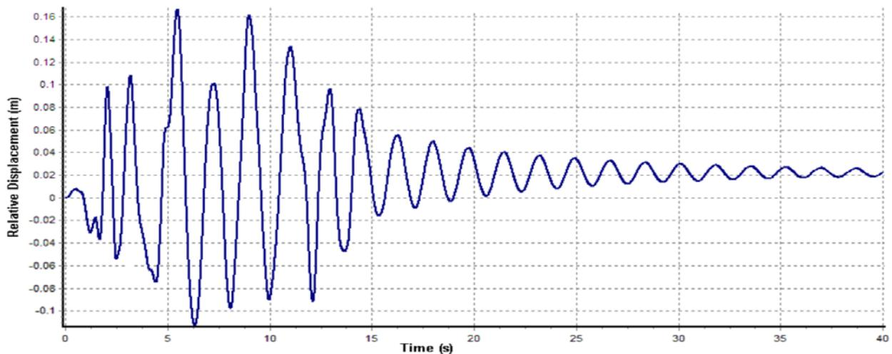
Fig. 3 Tip deflection response of original structure
