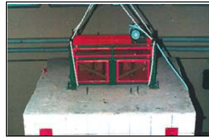
Fig. 7 Anchoring of the vibrodyne to the deck of the second floor
