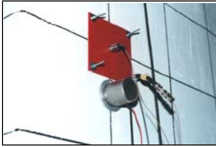
Fig. 10 A typical uniaxial accelerometer adopted in the present study
