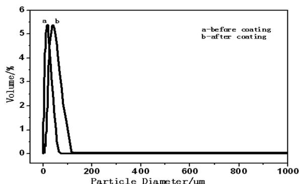
Fig. 5 Particle size distribution of ADN particles
