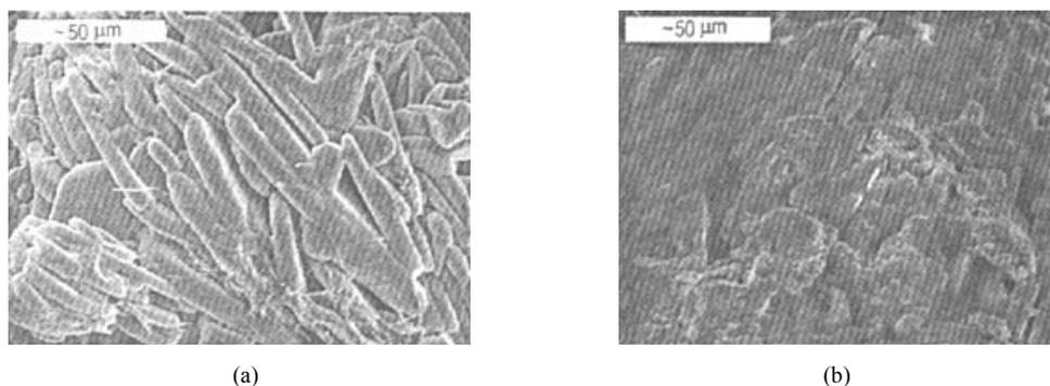
Fig. 4 Microstructures of ADN (×500, a: before coating, b: after coating)
