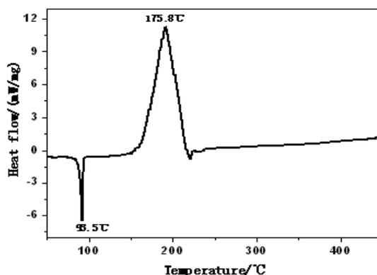
Fig. 3 DSC curve of ADN (heating rate: 10 K·min<sup>-1</sup>)
