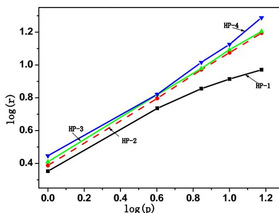
Fig. 6 Effects of different contents of ADN particles on the burning rate of the propellants
