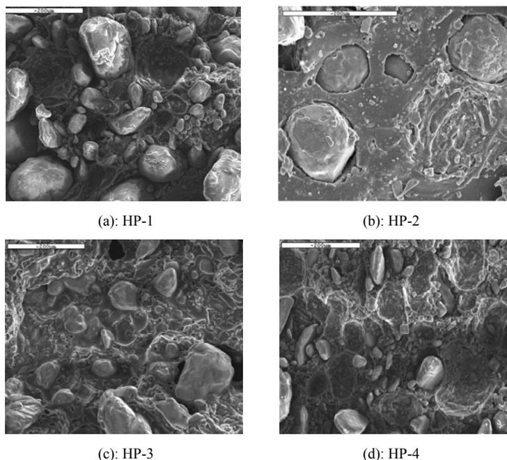
Fig. 6 Microstructures of HTPB-based composite propellant with and without ADN ( $\times 300$  multiple)
