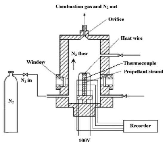
Fig. 1 The apparatus of chimney-type strand burner with observation windows<sup>[32]</sup>
