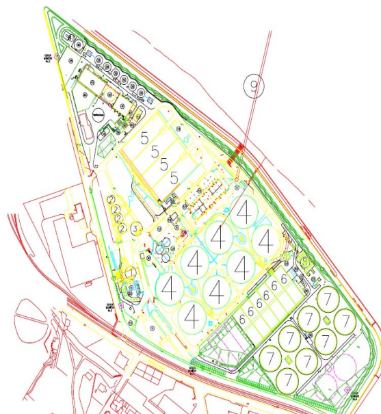
Fig. 5 Layout of Seafeld wastewater treatment plant: 1 is the screen house, 2 are the detritors, 3 Grit washing mechanism, 4 sedimentation tanks, 5 storm tanks, 6 aeration tanks, 7 final settling tanks, 8 UV treatment unit, 9 outfall tunnel
