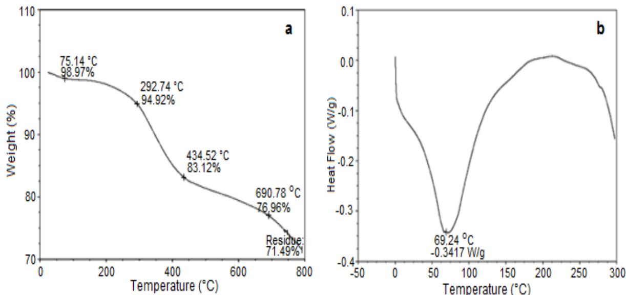
Fig. 6 (a) TG and (b) DSC curves of silver nanoparticles synthesized by reacting  $\text{AgNO}_3$  with Ricinus leaf extract
