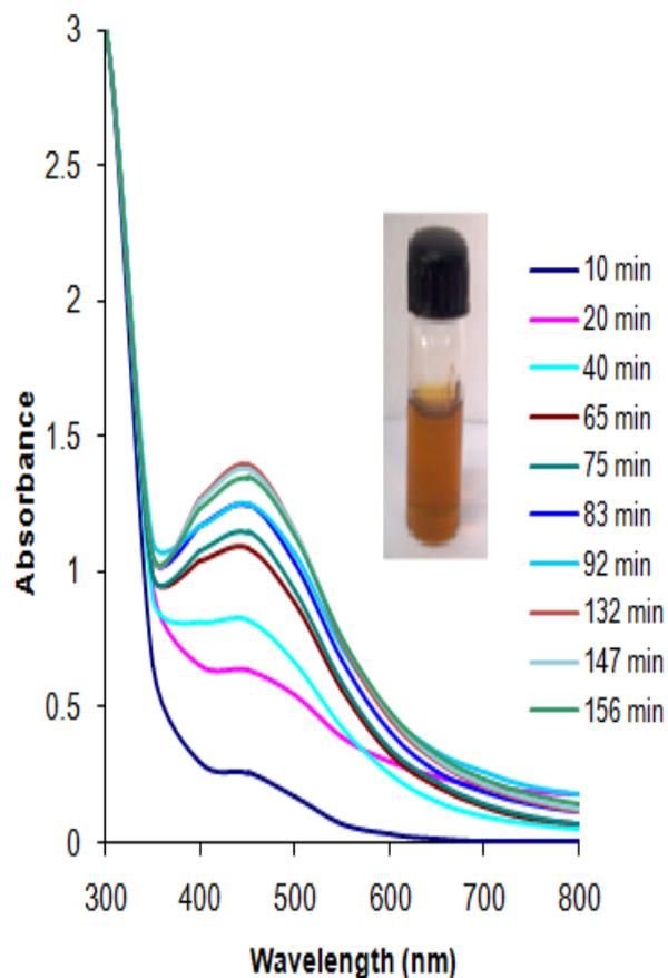
Fig. 1 UV- Vis spectra of nanoparticles measured at the time of reaction of *Ricinus communis* leaf extract with aqueous solution of 1mM  $\text{AgNO}_3$ ; the inset is synthesized Ag nanoparticles showing brownish red color after 3 h of incubation
