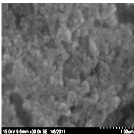
Fig. 3 (a) SEM micrograph of silver nanoparticles formed after reaction of leaf extract with 1mM AgNO<sub>3</sub> for 3 h
