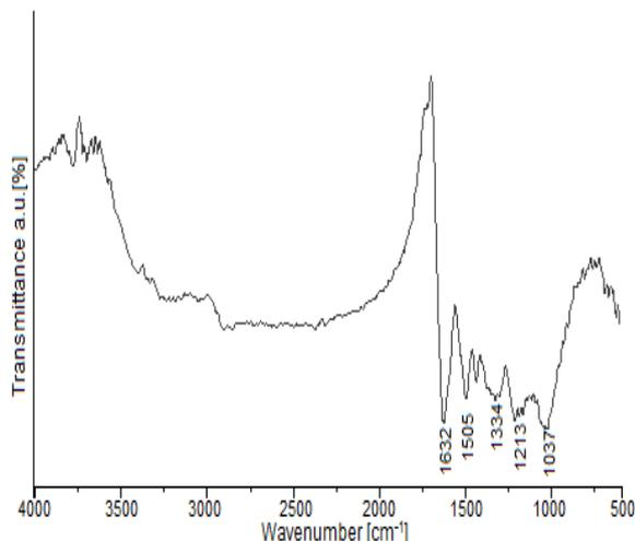
Fig. 5 FTIR spectrum of Ag nanoparticles synthesized by reduction of  $\text{Ag}^+$  ions by *R.communis* leaf extract
