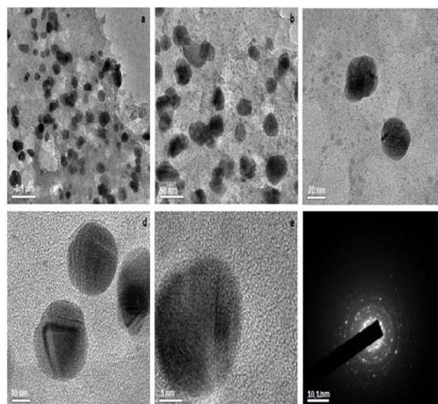
Fig. 4 (a-e) TEM images of silver nanoparticles at different resolution (f) SAED pattern
