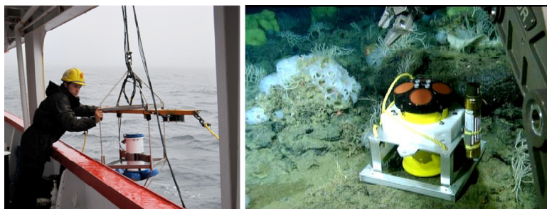
Fig. 3 Surface mounted (l) and bottom mounted (r) ADCP devices
