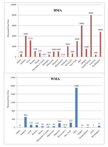
Fig. 7 Comparison of WMA production with HMA in cold region states [31]
