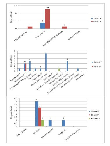
Fig. 8 Reduction in mixing temperatures achieved by using WMA compared to HMA [31]
