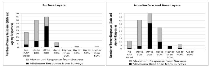
Fig. 9 States and agencies using RAP in surface and non-surface hot-mix asphalt pavement by percentage of RAP [39-41]
