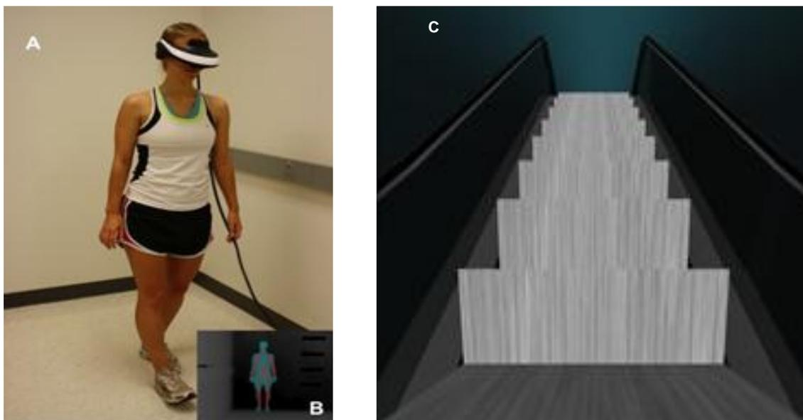
Fig. 1 Experimental setup with subject stepping forward (A), Xbox Kinect recording (B) and virtual environment projected in the 3D helmet (C)
