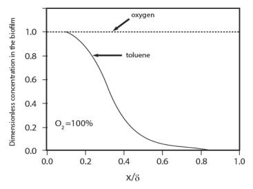
Fig. 5 Model predicted concentration profiles of oxygen and toluene in the biofilm at the middle point of the biofilter for inlet toluene concentration of 10.0 gm<sup>3</sup> and 100% oxygen
