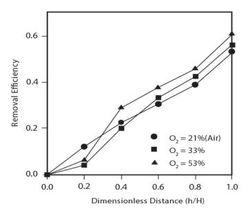
Fig. 2 Removal efficiencies at different oxygen contents (21%, 33%, and 53%) and for toluene concentration of 1.5 gm<sup>-3</sup>
