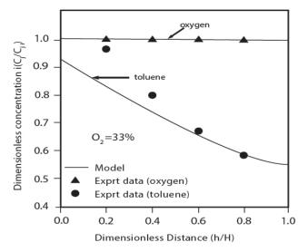
Fig. 3 Comparison between model-predicted gas phase toluene concentration and experimental data along the biofilter [oxygen content = 33% and  $C_{Ti} = 1.5$  gm<sup>-3</sup>]
