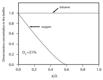
Fig. 4 Model predicted concentration profiles of oxygen and toluene in the biofilm at the middle point of the biofilter for inlet toluene concentration of 10.0 gm<sup>-3</sup> and 21% oxygen
