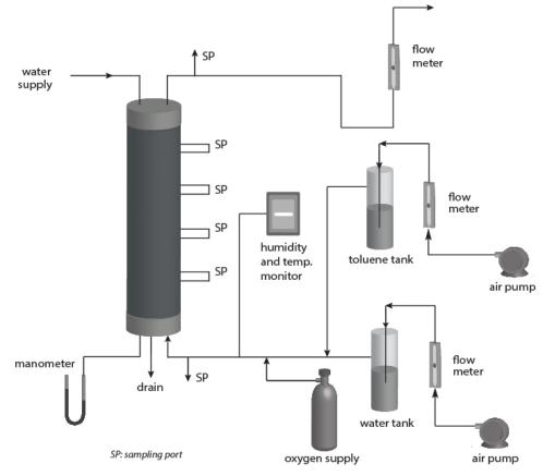
Fig. 1 Schematic of the experimental setup used in this study
