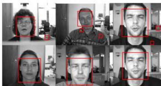
Fig. 10 The examples of the test images show faces are detected. With the small rectangles the top three images however show false positive detections in single image while in the bottom three images, detection of faces are done perfectly.
